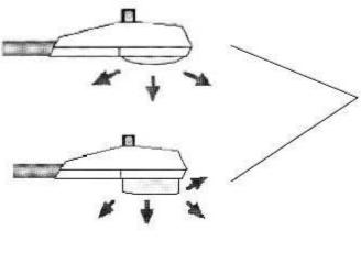
Partially shielded lamps—notice that the lens cover is visible when viewed directly from the side.
