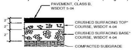
NOTE: DEPTHS ARE COMPACTED THICKNESS
